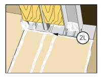
M. **If using sill nosing with a step down,** Install the sill pan and sill nosing into the opening. Press down to seal them into the opening. DO NOT overlap.
